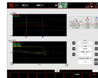
Temperature and compensation are displayed on MAZATROL SmoothG screen. Operator can adjust compensation by looking at the data.
